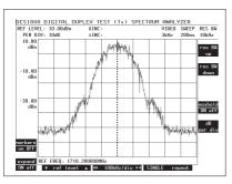
The tracking generator facility (with offset tracking) is provided for RF module characterization. With a useable frequency range of 100 kHz to 1 GHz and 1.3 GHz to 2.2 GHz, the spectrum analyzer supports IQ modulator alignment and the testing of internal local oscillators and IF systems. IQ alignment tests are recommended on most popular GSM terminals.
